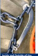
4A. Connect fastener on inside the tire. Count the same number of links on the outer side chain and place end of fastener through that link.
