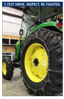
Test Drive, Inspect, Re-Tighten tire chains by REPEATING STEPS 4A- 4D so chains fit snug around the tire. Make sure the quick hook and fastener are
