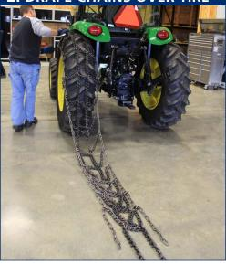
Drape chains over tire in the same position making sure ends of cross chain hooks face up and away from tire. Center chains on tire and position them to touch the ground in front of the tire. Tuck first cross chain under tire a bit in preparation to roll over them.
