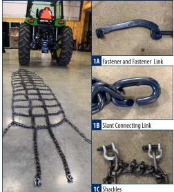
Lay chains out flat behind tractor making sure ends of cross chain hooks are facing up. Remove all twist and tangles.
