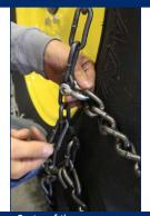
4C. Pull tail chain to tighten. Connect shackle on tail chain to side chain.
