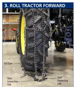
Roll equipment forward until the end of the chains are at a good working height—approximately axle height.
