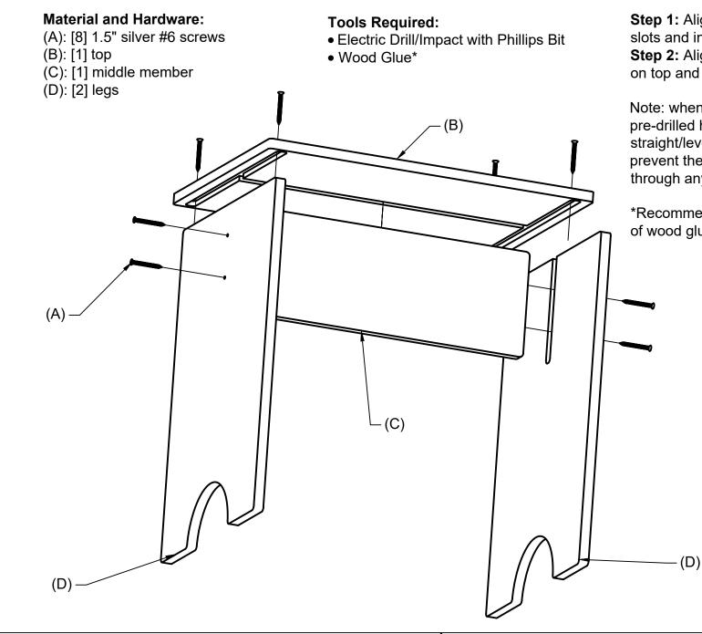
Step 1: Align center with legs 1 and 2 slots and insert (4) screws.Step 2: Align lower assembly into slots on top and insert (4) screws.
