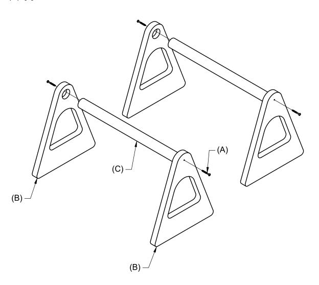
**Step 1:** Place (B) end plate on ground with hole facing up and insert small amount of wood glue.
