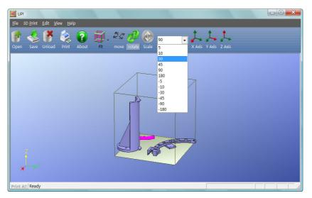
**Scaling the model:** Click "Scale", choose or input a scaling factor in the text box, and then either scale the model uniformly by clicking the scale button again, or choose the axis around which you want to scale if you only want to scale in one direction.
