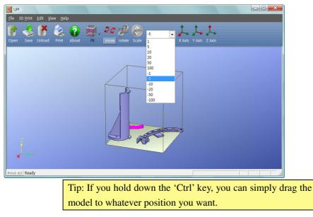
**Rotating the model:** Click the "Rotate" button on the toolbar, choose or input how many degrees you want to rotate in the text box, then choose the axis to rotate around.
