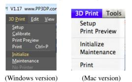
**TIP:** If your printer is not responding properly, the first thing to try is to re-Initialise the printer by clicking the 'Initialise' option from the '3D Print' menu. If still not working switch off and on the printer at the back. Check the printer drivers trouble shooting section. The printer can also be Initialised by pressing the front switch on the printer.
