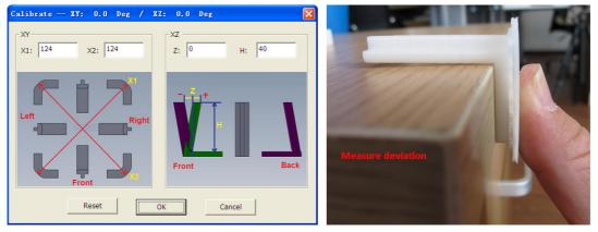
**IMPORTANT NOTE:** Before you enter any new calibration values, always click the "Reset" button, otherwise the new values get added to the old ones. Before you enter any new values, the bar at the very top of the screen should read: XY: 0.00 deg / XZ: 0.00 deg.
