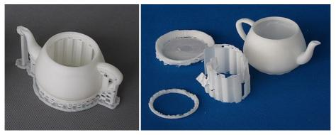
Printed models are composed of two parts. One part is the model itself, and the other part is the support material used to support any overhanging parts of the model.
