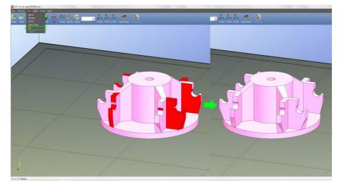
Merging models: Several separate models can be merged into a single file by using the "Merge" option from the "Edit" menu. Simply open all the models you want to merge and arrange them the way you want on the platform and click on the "Merge" option. When you then save the file, all the components will be saved as a single STL file.
