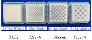
The easiest way to calculate how much material will be used for your model is to use the "Print Preview" option under the "3D Print" menu. This will tell you the total weight of material used,
