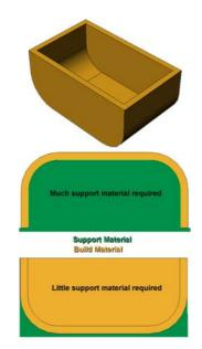
**Support - Dense:** This represents how many layers of 'solid' (dense) material form part of the support structure directly beneath the model.  $Default = 3 \ layers$
