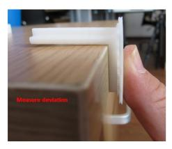
Remove the Front Centre 'L' shaped component, and measure its deviation. Put the exact value into the Z box. If it deviates to the right side, the value to be put into the Z box will be a positive value. If the deviates to the left, the value to put into the Z box will be a negative value.
