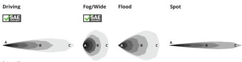
A - lux at 10 meters B - Distance (m) with 1 lux C - Distance (m) with .25 lux
