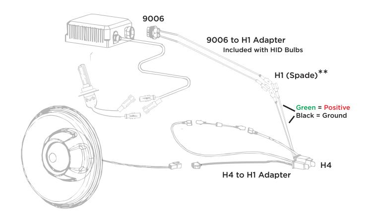
\*\*Be sure to wire and secure properly with electrical tape or shrink wrap.
