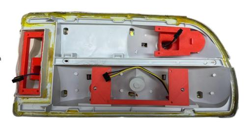
Plug in the wires into the boards.
