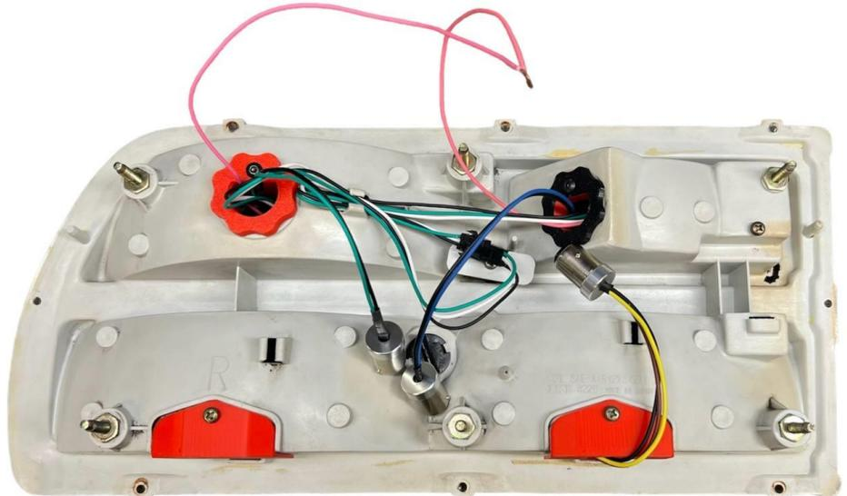
At this time, the board can be placed back into the vehicle to program or connect to a separate power source to program before placing it back into the vehicle. Proceed to [Sequential Lighting Operation](#): on page 9.
