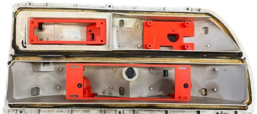
Attach the end caps on the backside of the housing and securely fasten with the included M3x8 screws.
