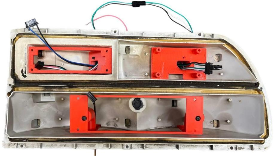
Plug in the wires into the boards. For the reverse and turn signal boards, the plugs can be inserted into either slot on the board.
