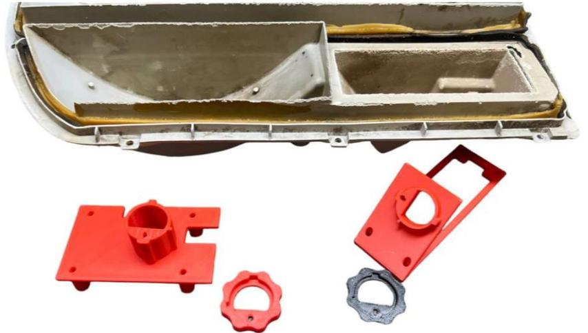
Place the brackets in the corresponding light cell in the orientation shown. They should fit in very snug.
