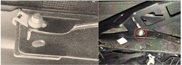
3: Next, install the 6mm carriage bolt and nut on the end slot securing to the bumper. (Pictured below) As previously stated, take out the slack but don't completely tighten the bolts down yet.
