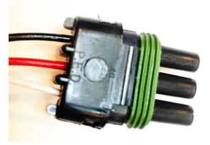
You can now install these on your bare light wires. BE CAREFUL to MATCH the colors up in alignment to your connector wire colors on your harness!! If you don't match the colors up, you will either blow a fuse, or the lights will NOT WORK. It isn't the lights, it is your alignment.
