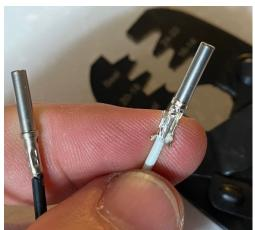
Slide the wires into the new plug as shown. Just like the 2 way plugs, they will slide into the slots until they click into the clips. Make sure they are securely in the clips. Then, snap the 3 way orange cap on the end. Pay attention to which color wires you put in which hole so you don't short them out.
