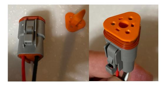
Last, put the other ends on your lights themselves. The opposite ends are similar. The pins don't have a barrel though. They have a slim pin. Apply them with crimpers the same way as the others. Slide them in and make sure they click into the clips in the plug. Instead of an orange cap, you have a green snap in plug that goes in the middle between the pins in the hole.
