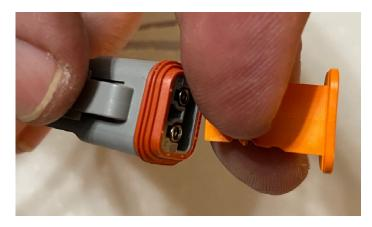
Next, notice the 2 clips inside. You will use a small screw driver or pic and pull those back. Then, you can pull the pins out the back side.
