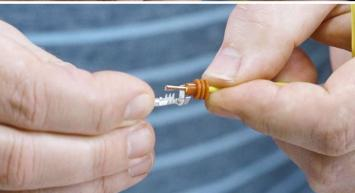
Now, place the wire into the pin receiver. Make sure the skinniest part of the orange rubber seal is set between the two large fins and the bare wire is set in the ribbed section of the pin.
