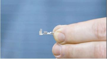
Both pin types have the same opposite ends with two sections that will need to be crimp down.
