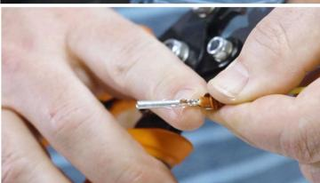
First, crimp down the ribbed section onto the bare wire.
