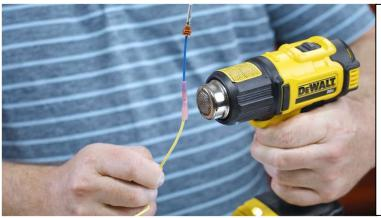
Next, use a heat gun to melt the end to make a tight seal.
