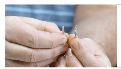
There are two different type of connector pin ends.
