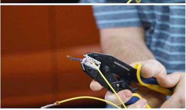
Now, take your crimper tool and crimp down the metal section securing the bare wire.
