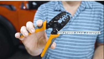
A weather pack crimper will make crimping the pin sections down much easier.
