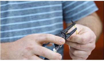
First, you will need to cut and strip about 1 / 4 inch of the rubber tubing revealing the bare wire.
