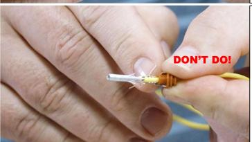
DO NOT push the bare wire all the way up inside the pin.
