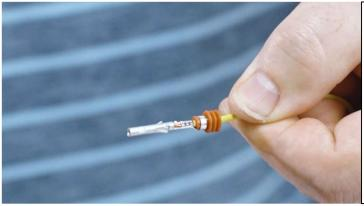
Next, crimp down the two large fins around the orange rubber seal.
