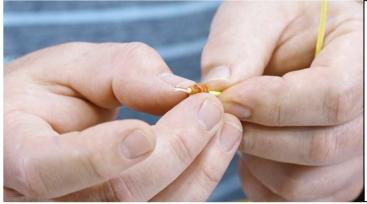
Next, slide an orange rubber seal over the copper wire. Make sure the skinniest portion is closest to the exposed wire and it is lined up the end of the rubber tubing of the wire.
