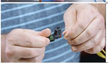
Next, place the assembled pin into the bottom of your connector.
