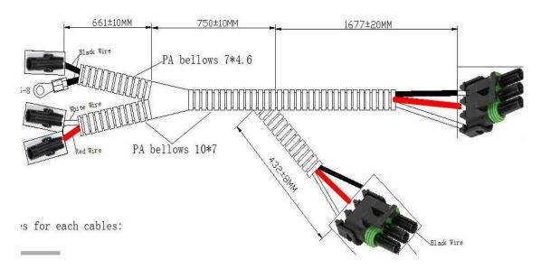
Each one INCLUDES sets of the connectors below. Singles go on the switch wires or trigger wires.
