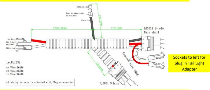
Each one INCLUDES sets of the connectors below. Singles go on the switch wires or trigger wires. The 3 way goes on ANY light that doesn't have a plug on them.
