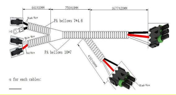
Each one INCLUDES sets of the connectors below. Singles go on the switch wires or trigger wires.
