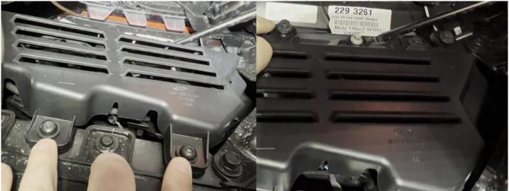
2: Once you remove those, the Fog Housing will dangle by 2 more bolts that were HIDDEN under that cover on the top portion. You can remove those 2 bolts, and the housing should come right out. At this point, you will also want to disconnect the factory fog connector plugs as well. The red clips need slid back to press and release. They are LOCKS.
