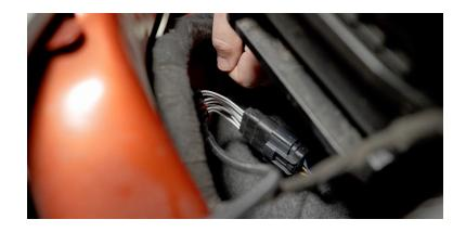
Next, run the long end of the headlight marker adapter along the top of the grille area where the plastic cover was. Follow the GROOVE.
