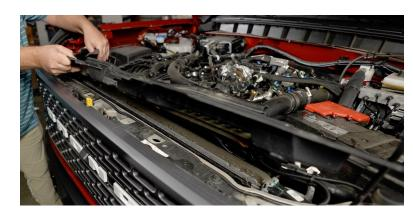
Make sure to lift the plastic piece attached to the airbox that sits on top of this plastic cover to slide the cover out.
