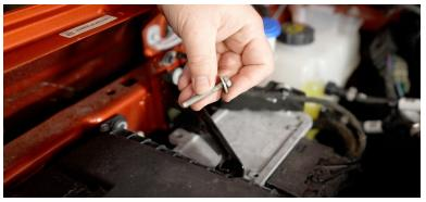
You can lift the airbox out of the way enough to get access to the headlight connector.
