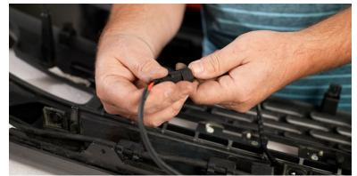
Next, attach the grille back onto the Bronco. Make sure the long end of the marker harness is fed out to the top of the grille, on the driver's side.
