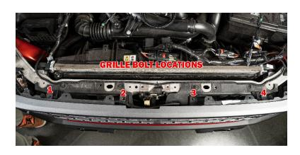
After these screws are taken out, you can now pull the grille free. There are several clips holding the grille on.
