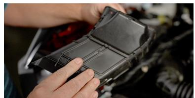
Now, you can remove the bolt holding the airbox to the Bronco.
