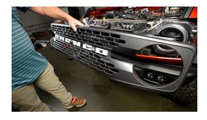
On the back side of the grille, you will find a plastic back panel. This panel has 6 screws along the top and 2 screws holding the camera in place.
