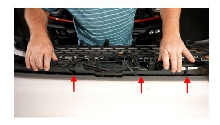
Make sure to NOT tighten the screws down too much in which it can put a lot of pressure on the wires.
