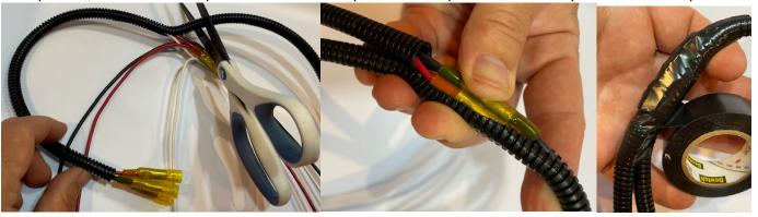
Then run it the rest of the way up EXCEPT the last 20" of the black wire. Keep that one out of the loom and wrap tape around it to secure it there. Once you're finished, your harness should look like the bottom right photo. The end with the ring terminal, pink and blue connectors go to the switches. The other end goes to the fogs. The short end is the passenger side.
