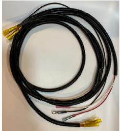
When connecting the fogs, combine ALL 3 reds into the RED harness wire. Combine all 3 Black ones into the black harness wires and all 3 White ones into the white harness wires on each side.
