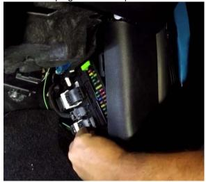
**Step 2:**Remove the red clip CAREFULLY from the bottom of the plug. Be careful not to break off the tabs on the end.
