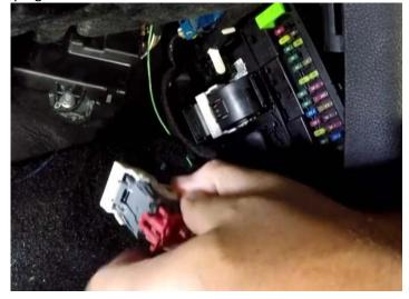
**Step 3:**Remove the zip tie from the top cover and remove the cover. Then insert the pin in the SECOND from the right hole from the backside of the plug on the top row. See pic with it being pointed to. DO NOT FORCE. If it is difficult going in, it's upside down. The FLAT part is the top.
