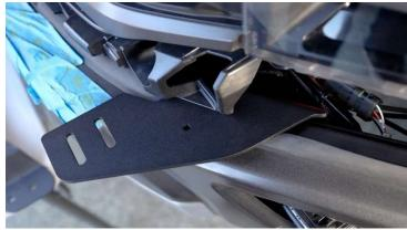
Next you will need to attach the bumper stop (C) on the bottom of the Main Mount between the bumper and mount at the center hole. And use the push pin to attach from the top.
