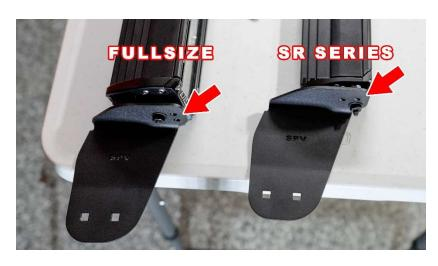
The Rigid Adapt Light Bar uses the long nose mount. The best bolt locations for the Adapt is the middle hole and front slot. The slots are used for angle adjustments.
