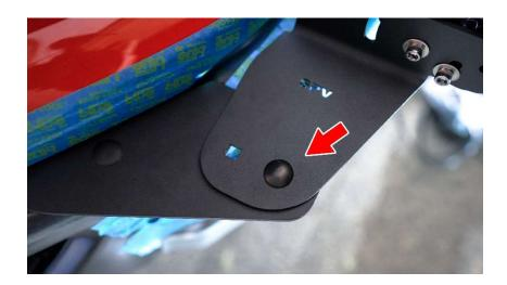
After installing the mounts on your choice of light bar, line up the square holes with the slots on the Main Mounts. Use hardware E to attach each side to the main mounts. Each side uses 2 bolts and 2 locks nuts.
