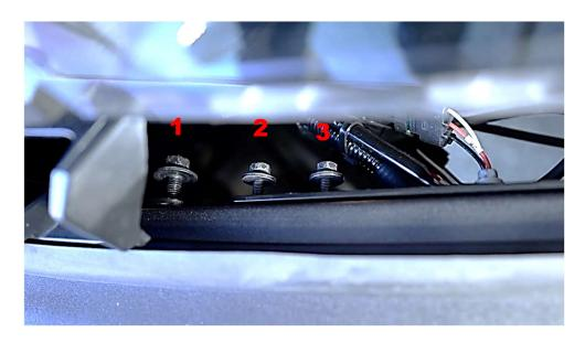
The back cover on Bolt(2) will need to be pulled back and will sit on the backside of the bracket. This bolt will need 2 spacer washers (A) if you have the factory fogs. These washers will go where the cover tab was originally. If you do not have fog lights, bolt(2) and bolt(3) will need one spacer washer each. Don't tighten all the bolts down until you adjusted the mount the way that best suits your needs.
