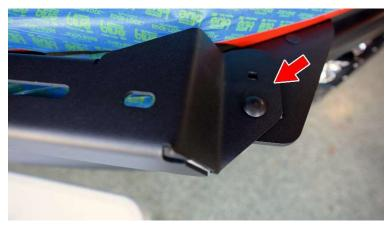
After installing the main mounts, place the Universal Cross Mount across the top of the bumper. Line up the square holes with the slots on the Main Mounts. Use hardware E to attach the cross mount to the main mounts. Each side uses 2 bolts and 2 locks nuts.
