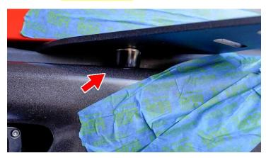
The bumper stop should rest on top of the bumper.
