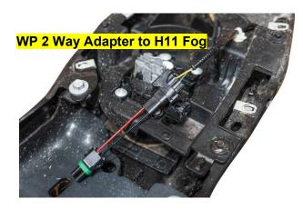
If you need to attach a splitter, connect it to the end of the corresponding adapter and then to your main power connector.
