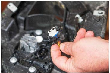
First, you will need to unplug the connector from the back of the light fixture.
