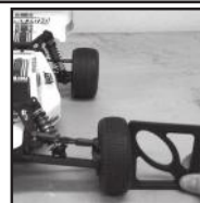
Testing camber with camber gauge
