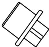
**STEP 1:** Attach a mouthpiece to the breathalyzer. It protects the sensor from droplets from the mouth, which could damage it. The mouthpiece also ensures a consistent blowing pressure, therefore contributing to a more accurate reading.
