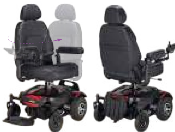
Very easy to convert from rear to front wheel drive: Just release and rotate the chair 180°
