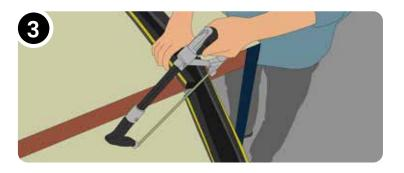
Use a hacksaw or utility knife to cut the wrap-around seal to size.
