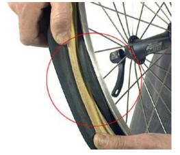
**Warning:** This picture shows a section where the innertube is between the bead and rim. If this occurs, pinch the tube and tire together with your fingers and work them around until the tube works its way back inside. *DO NOT use a tire lever or other object to "stuff" the tube back in.*
