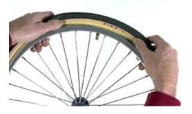
**Step 7:** After your tube is inserted into the tire, start at the valve hole again and begin working the remaining bead onto the rim. Ensuring that the bead is pushed tightly down into the rim as you go will make the final bead "pop" much easier.
