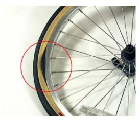
**Warning:** This picture shows the innertube beginning to bulge out from under the tire after inflation. About 5 seconds from this point, the innertube will expand quickly out, lifting the tire off the rim before blowing. Most high pressure tires have enough pressure to blow the sidewall out of a brand new tire, so inflate your tires slowly to their *recommended* pressure while looking for areas where the tire is not seated properly on the rim.
