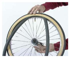
**Step 4:** After half of your tire is installed, lift the uninstalled bead at the valve hole and insert your innertube's valve stem into the rim. If necessary, tuck the base of the valve stem into the tire.
