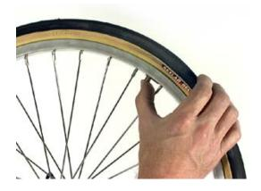
**Step 10:** Before inflating the tire, push the valve stem into the tire to ensure the valve base is inside the bead. If you don't the innertube will lift the tire off the rim as you inflate it.
