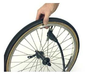
**Step 12:** Inflate the tire until it begins to take shape and firm up slightly (10-20psi). You are trying to help the innertube seat itself inside the tire.
