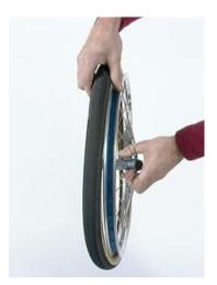
**Step 2:** Starting with the tire alone (no tube), line up the decal on the tire with the valve hole in the rim. Some cyclists like to align the inflation pressure information with the valve stem. Either way, if you always install your tires the same way, it will help you determine the puncture location in the event of a flat tire.
