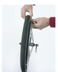
**Step 3:** Starting at the valve hole, slide one side of the bead over the lip of the rim. Hold the tire in place at your starting point with one hand, and use your other hand to work your way around the rim, pushing the bead over the rim as you go.
