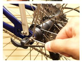
Attach and tighten the looped ends of the fender braces to the bicycle frame mounts with a 20mm allen bolt and a 6mm washer. One bolt will hold both fender braces on a side. **NOTE:** *Be sure the drive-side bolt does not protrude past the inside of the dropout. If the end of the bolt extends into the driveline, the chain could hit the bolt when you shift into your smallest cog. Add washers or source a shorter bolt so the end of the drive-side bolt is flush with the inside of the dropout.*
