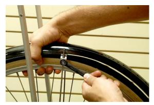
Now press the top of the fender down to match the profile of the tire. Hold it in place and tighten the two top mounting locknuts. Be sure both sides are even and that there is no tire contact.
