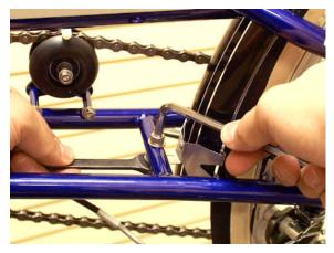
Start with the rear fender. Attach the forward mounting tab to the frame with the 30mm Allen bolt, two 7mm washers and a nylon locknut. Tighten straight and secure.
