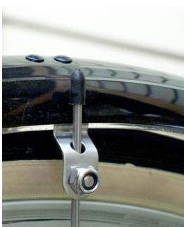
Your fenders are installed! Take the black rubber caps and press them onto the tips of the fender braces to protect your clothing and skin from sharp edges. It should be unnecessary, but you may trim any excess fender brace with a grinder if desired.
