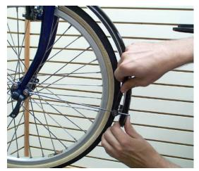
Attach the two **rear braces** to the **rear mounting tabs** on the bike's fork with the remaining two 15mm allen bolts and 6mm washers. Press the rear of the fender down to match the profile of the tire. Hold it in place and tighten the two rear mounting locknuts. Be sure both sides are even and that there is no tire contact.
