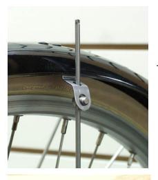
Thread the fender braces through the mounting tabs as shown (left).
