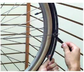
Slide the tail end of the fender on the braces until the arc of the fender matches the arc of the tire. Hold the fender in place and tighten the two rear mounting locknuts. You may need to flex the fender to match the tire profile correctly.
