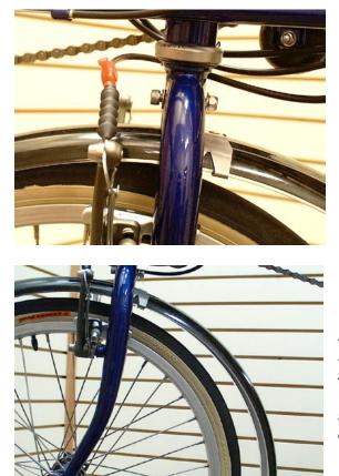
Moving to the front of the bike, attach the front fender to the hole in the top of the fork with the 40mm allen bolt, two 7mm washers and a nylon locknut. The long half of the fender should be to the rear of the bike. Be sure there is no brake interference and tighten securely.
