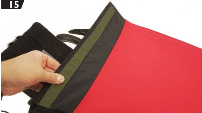
Fig. 15: The wind deflector is held in place by a flexible metal strip. Make sure that this metal strip is in the correct position before starting your ride (see image).
