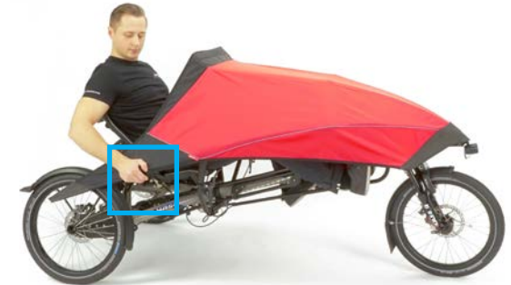
Fig. 6: Guide the coupling plate of the Foldable Fairing into the U-tube from above.
