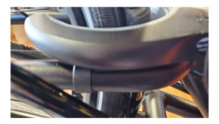
Open the Cateye Clamp package and install one clamp on each side of the chainstays in the area of the rear wheel (the included hardware and shims in the Cateye packages are not needed). Place the lock on top of the clamp, aligning the lock hole slots with the clamp hole .
