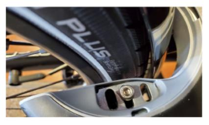
Thread the two long bolts through the lock slots and Cateye Clamps on each side of the trike, as shown in the photo. Be sure everything is aligned properly, so the lock will close.
