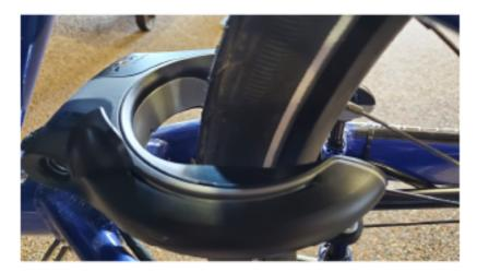
Secure the black lock cover onto the top of the lock. It will just snap into place.
