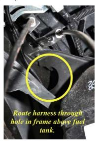
iii) Secure the bed light LED wire harness to the OE harness in front of the fuel tank using wire ties. (Fig. 3-4)
