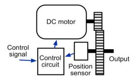
A DC motor (normal motor that can rotate continuously) is attached to a gear box, which drives the servo arm, but is also coupled to a position sensor that provides feedback to an electronic control circuit that keeps the servo arm at the correct angle.
