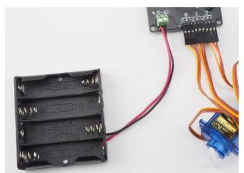
Using a screwdriver, unscrew both of the terminals in the terminal block and then insert the end of the red lead into the screw terminal marked with a + and do up the screw of the terminal. Do the same with the black lead in the terminal marked with a -.
