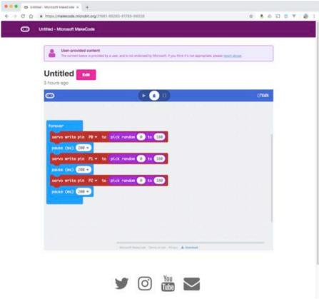
Click on the *Download* link at the bottom of the window and copy the HEX file onto your micro:bit. Once flashing is complete, the servomotors should spring into action moving by random amounts.
