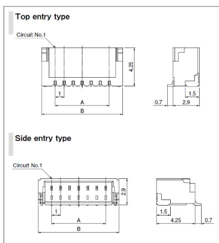
The following PCB footprints show the pin numbering for both top and side entry types and signal direction from the target perspective. For clarity, the fact that we are showing UART on a side entry type and serial debug on the top entry type is just for example – either type can use either interface:
