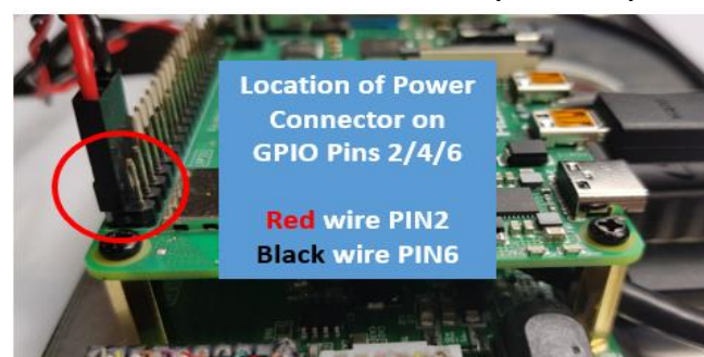
Item #5 – Internal Power Connector (Side view)
