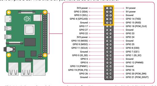
**Note:** This MaticControl module covers the pins for: 5V power supply, GPIO15 (RXD) and GPIO14 (TXD). If you want to use them, we offer modules (HATs) that provide access to these pins via separate connector on the top of the board. **For more see LeapMatic.com**
