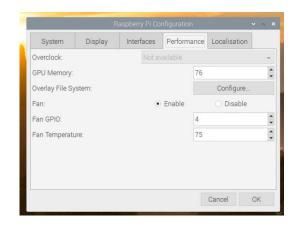
Thus, when the processor reaches the temperature you set, the fan will turn on. It will turn on off only when the processor temperature drops 10 degrees below the set on temperature. (For example, if you set the On temperature to 75 degrees, the fan will turn off when the processor reaches 65 degrees). With these few easy steps, you now have automatic fan control.
