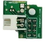
Place it on pins 1-8 and connect your fan to the connector on the top. And this is all you have to do on the hardware.
