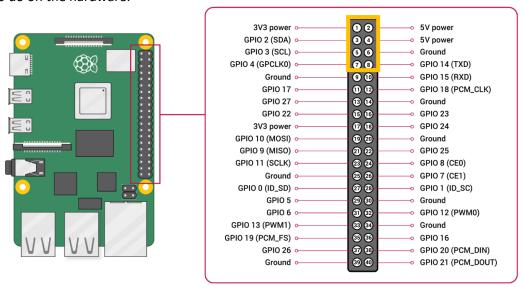
**Note:** This MaticControl module covers the pins for: 5V power supply, I2C, GPIO15 (RXD) and GPIO14 (TXD). If you want to use them, we offer modules (HATs) that provide access to these pins via separate connector on the top of the board. For more see LeapMatic.com
