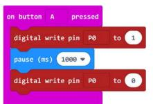
In this simple program, pressing Button A on the BBC micro:bit will set the output of Pin 0 to be 'High' for 1000ms (1 second), and then set it back to 'Low'.
