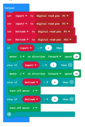
The example blocks (left) cause both motors to move forward with pins 1 and 2, and uses the button inputs at pins 5 and 11 to stop each motor separately.
