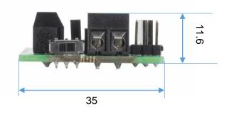
The PCB is 1.6mm thick
