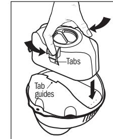
Align the FROG @ease SmartChlor Cartridge with tab guides on the FROG @ease Mineral Cartridge. Push together until you hear the cartridge click into place.
