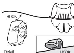
If only a small amount is left attach a new FROG @ease SmartChlor Cartridge and hook the old cartridge on the tether until it is completely empty.
