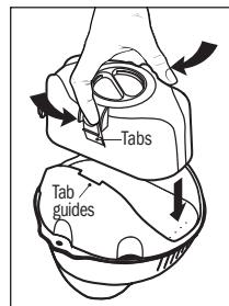
When the product flips over, the FROG @ease SmartChlor Cartridge is empty. Remove the empty FROG @ease SmartChlor Cartridge and replace with a new one.
