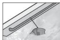
This system naturally sits at a tilt in the water. To check if the FROG @ease SmartChlor Cartridge is empty, lift up and drain all the water from the system. You should be able to tell by looking if there is still FROG @ease SmartChlor left in the cartridge.
