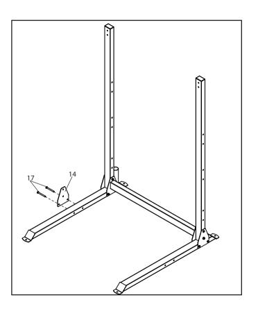
Attach the Front Upright (4) to the Left Base with two M10x95mm Bolts (17) as shown.
