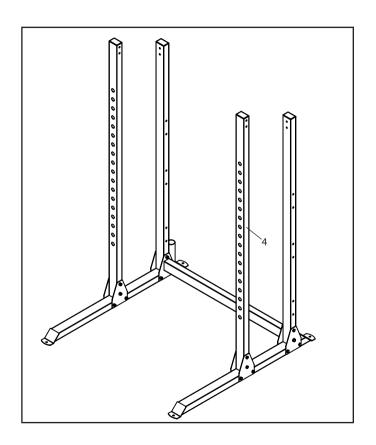
Orient the Crossmember (6) and Back Plate (13) as shown, secure with M10X70mm Bolts (16), M10 Spring Washers (19), M10 Washers (20) and M10 Nuts (18) as shown.
