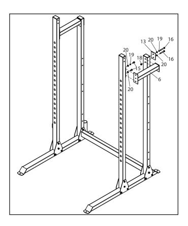
Identify the Pull-Up Bar (7) and orient as shown. Make sure that the long side of the bracket is in the indicated location.
