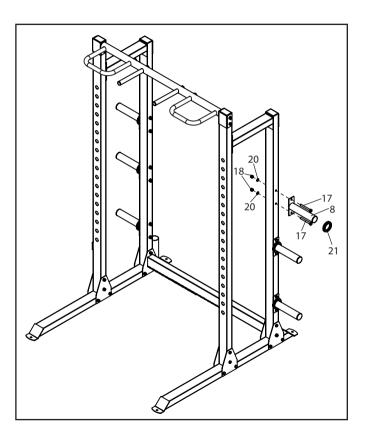
Insert the Right J-Cup (9) into the desired adjustment hole in the Right Front Upright (4). Then, insert the Right Spotter Arm (11) into an adjustment hole below the Right J-Cup. Repeat this step on the other side of the weight rack.
