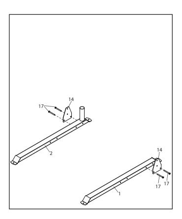
Attach the Rear Upright (5) to the Left Base with two M10x95mm Bolts (17), M10 Spring Washer (19) and M10 Washer (20) as shown.
