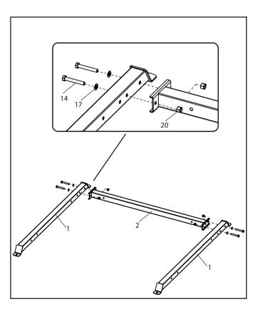
Attach one Support Plate (9) to the Base (1) with M10x70mm Bolts (14).
