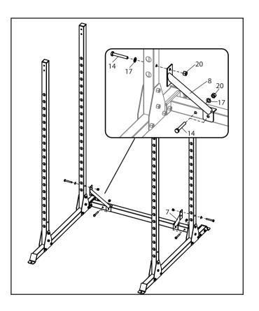
Orient the Crossmember (4) and Plate (10) as shown, secure with M10x70mm Bolts (14), M10 Spring Washers (16), M10 Washers (17) and M10 Nuts (20) as shown.
