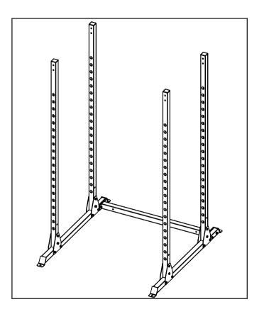
Orient the Left Support Frame (8) as shown, secure to the Upright with M10x70mm Bolt (14), M10 Washer (17) and M10 Nut (20).
