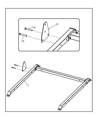
Put the Upright (3) on Base (1) as shown, insert two M10x70mm Bolts (14) into the holes.
