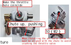
Installation to avoid excessive force fracture
