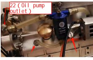
21 (Connect oil pump inlet after installation)
