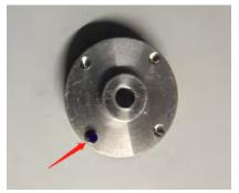
Just install a magnet in any mounting hole. It needs to be pressed in with a tool magnet. Or use a drill to enlarge the hole diameter, and then use glue to stick it
