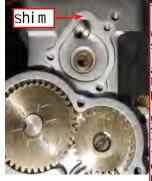
The pulley is fixed with high-strength 271 anaerobic adhesive. Fix the pulley note: the pulley groove should be flat with the crankshaft pulley
