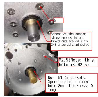
The starting motor screw shall be put in before installing 41 (screw No.: 1)
