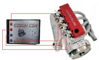
If there is no series resistance between the high voltage wire and the spark plug of CDI, the noise that interferes with the sensor may be generated, causing four high voltage wiras to generate eparks at the same time, But this will not affect the operastion. But I suggest you connect the resistance we provide in series between the end of the high-voltage wire and the spark plug
