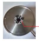
The tension sleeve and flywheel shall be kept flat as far as possible
