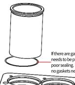
If there are gaskets on the cylinder liner, only one gasket needs to be placed, as excessive placement may lead to poor sealing. If there are no gaskets present, it means that no gaskets need to be installed
