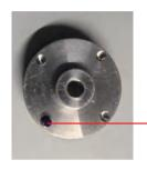
After you receive the CDI igniter, there is a very small magnet in the package. Please note that there are colors on one side of the magnet, and those with colors are installed outward, as shown in the figure
