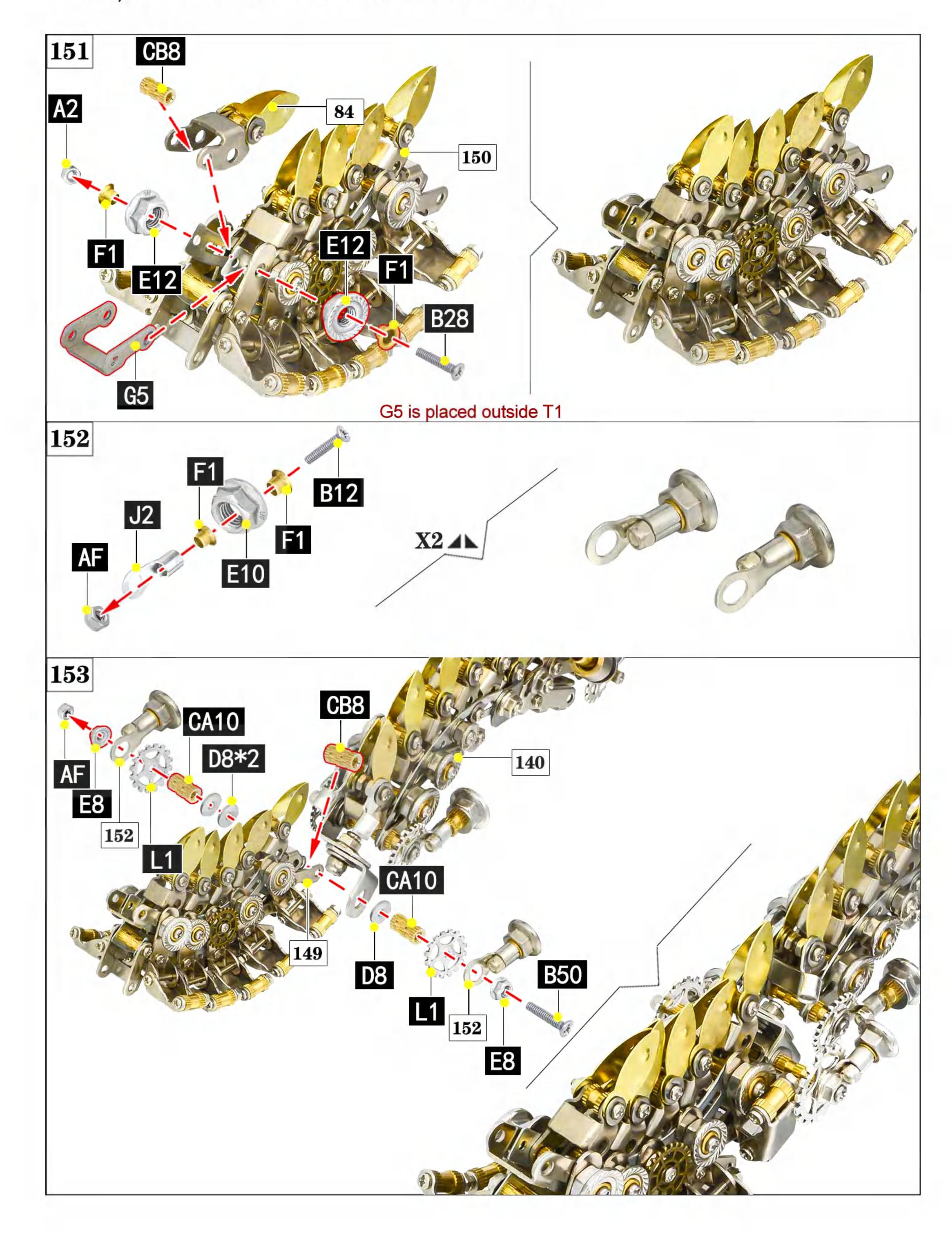
Assembly skills, screws are preferred. (X2 ◢▶)Means: assemble 2 and horizontally symmetrical.
