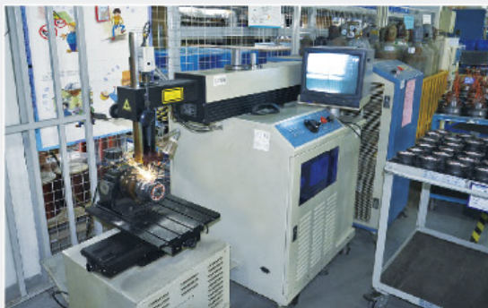
Automatic Laser Welding
