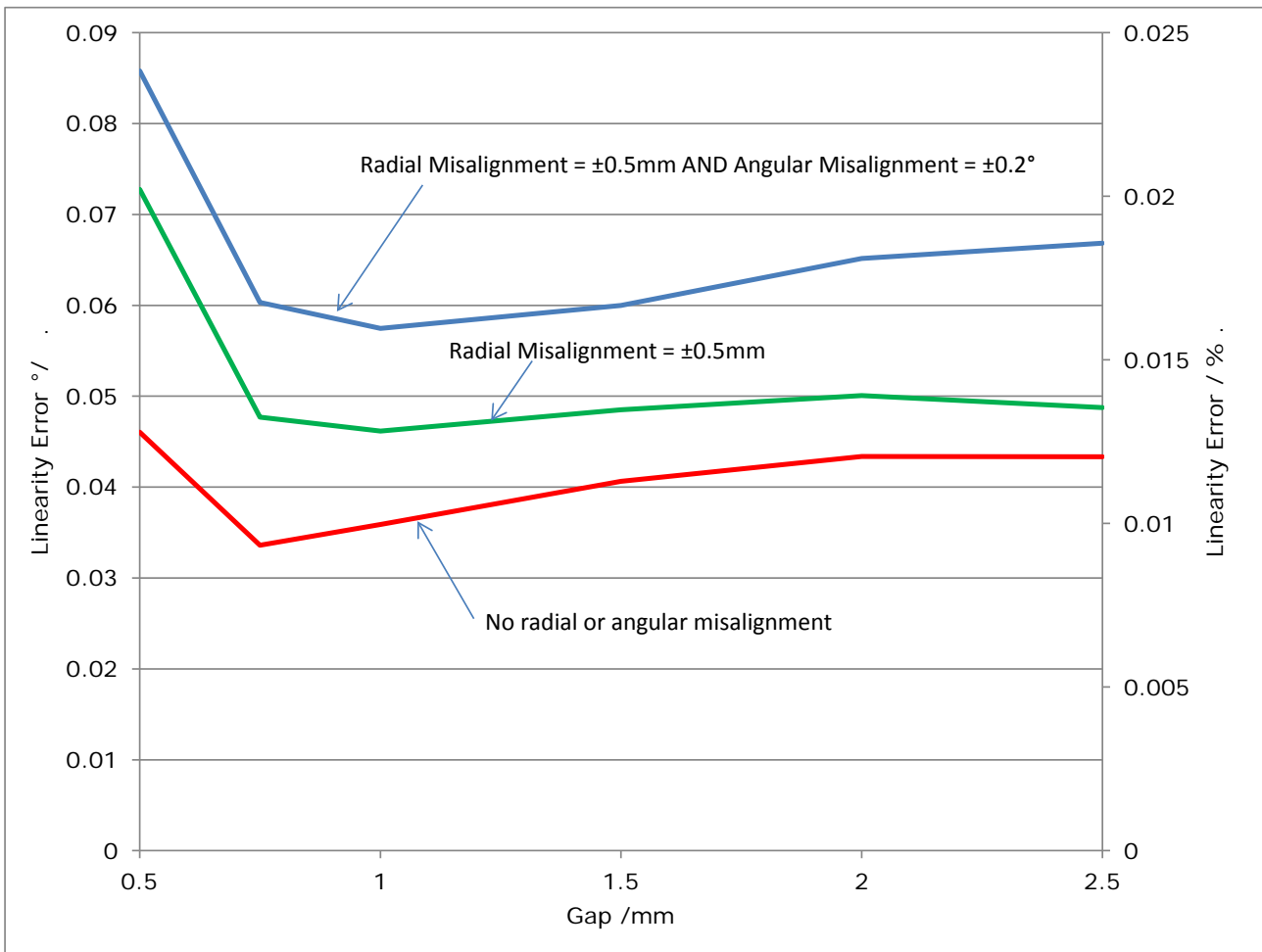
Figure 15 Linearity Error as a function of Gap and misalignment, free space
