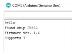
Bring your NFC/RFID tag or card close to the selected antenna. You can read the information in the serial monitor.
