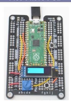
It can be tricky to work out which pin is which when using a Raspberry Pi Pico with prototyping board. The MonkMakes Pico Proto PCB solves this problem by labelling the Pico pins on the PCB.
