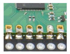
You can also solder your Pico to the PCB using header pins that are first soldered to the Pico and then to the Pico Proto PCB, but make sure you have the Pico Proto PCB the right way up, or the pin labels will be mirroroed.
