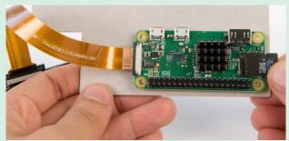
Insert the micro SD card into the silver socket on the Pi Zero – the metal contacts on the SD Card should face toward the green board.
