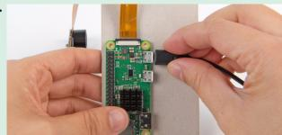
Power the assembled unit by connecting the USB power bank to the Pi Zero. The small end of the USB cable plugs into the 'PWR' port on the end of the Pi Zero closest to the camera. The large end of USB cable plugs into the USB battery (or any USB power source).
