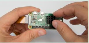
carefully stick the heatsink squarely over the large black chip on the Pi Zero.
