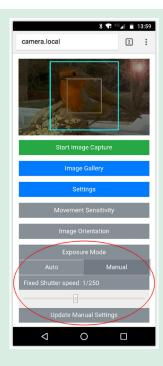
By Default, the My Naturewatch Camera is set to automatically control the exposure of the image. However the exposure can be set manually if the scene has mixed lighting conditions, or if you would simply like to modify the shutter speed to create different effects.
