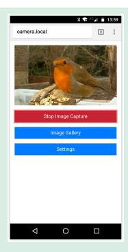
The My Naturewatch Camera takes photos by continuously monitoring the live preview feed for movement. When you want to begin this process, press 'Start Image Capture' button. The camera will now taking pictures automatically and the button will change to a red 'Stop Image Capture' button. All the recorded images will be stored within the Image Gallery. Press the 'Stop Image Capture' button to cease capture.
