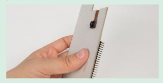
**Tip:** If you plan to use a large container, the Raspberry Pi and camera can all be mounted to one side of a piece of card.
