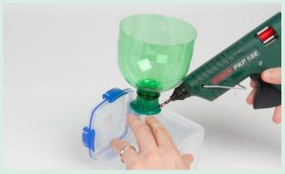
food storage box and make a waterproof seal using a hot glue gun, Sugru (<a href="https://sugru.com/">https://sugru.com/</a>) or household sealant.
