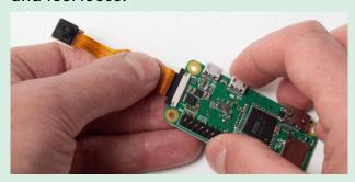
Now insert the camera module ribbon under the black strip and into the white
