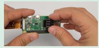
Raspberry Pi heatsinks generally have self-adhesive tape already applied. Peel away the protective layer of the tape and carefully stick the heatsink squarely over the large black chip on the Pi Zero.
