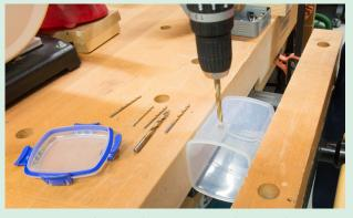
accommodates the camera lens. The hole should be about 10mm in diameter and is best made by starting with a small drill and progressively working up to the desired size in order to prevent the container from cracking.
