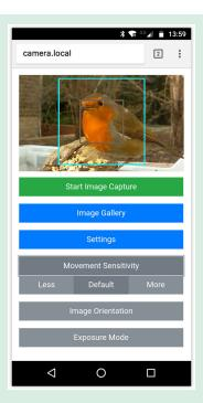
The My Naturewatch camera takes photos by looking for a significant change in what it can see. The square outlines on the preview image above represent the size of change the camera looks for to determine whether or not to take a photo. The sensitivity of the camera can be altered to prevent false positives – unwanted pictures taken when there is no wildlife in the camera frame.
