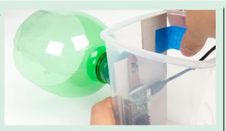
Tape the cardboard camera mount inside the container, with the lens positioned to look through the hole you drilled. Attach the battery pack.
