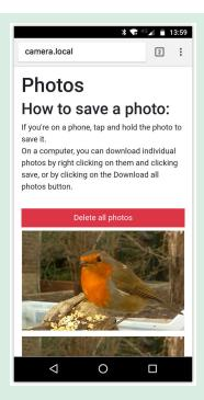
Pressing the 'Image Gallery' button on the main screen will lead to a new page showing all the pictures the camera has captured. On a phone, save photos by tapping and holding on them. Once you have saved the ones you want, delete the photos from My Naturewatch Camera by clicking the 'Delete All Pictures' button.
