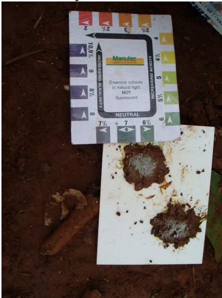
Photo 108: pH Field test kit.
